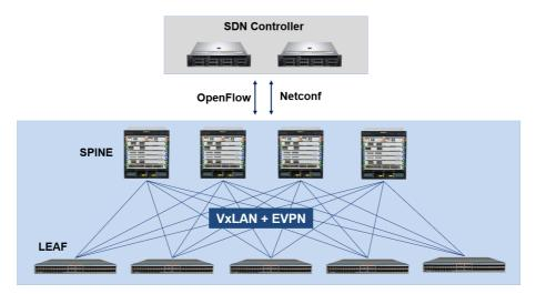
Fabric architecture has become a common and popular design option for building new-generation enterprise data center networks. Virtual Extensible LAN (VXLAN) and Ethernet VPN (EVPN) is essentially becoming the standard technology used for deploying network virtualization overlays in data center fabrics. NSS5950-32QFP switch support VxLAN and EVPN which is suitable to deploy in data center application.
