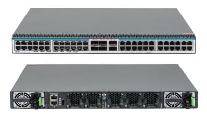
NSS5830-54XTQFP supports 48\*1/10G electric interfaces, 6\*40/100G QSFP28 optical interfaces, five modular fan slots, and dual modular power slots.
