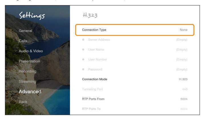
COLLABORATE® Live utilizes H.323 to transport video/audio via DNS and NAT addressing, and to communicate/interact with either a COLLABORATE® Central server or a standard gatekeeper server, one of which you can choose to work with in order to gain better performance and flexibility in point-to-point and multipoint videoconferences.
