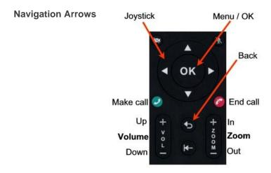
In addition to the navigation arrows, the following buttons are available around it:
