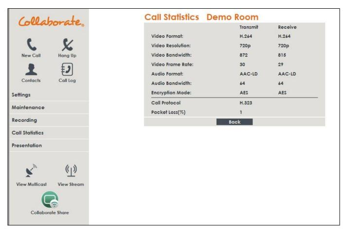
The image above confirms the Call Protocol, Video and Audio formats, Video resolution and frame rate, Audio and Video bandwidth, Encryption Mode, and Packet Loss details.
